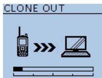
When the PC starts reading the data from the transceiver.
