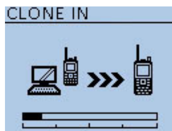
When the PC starts writing the programmed data into the transceiver.
